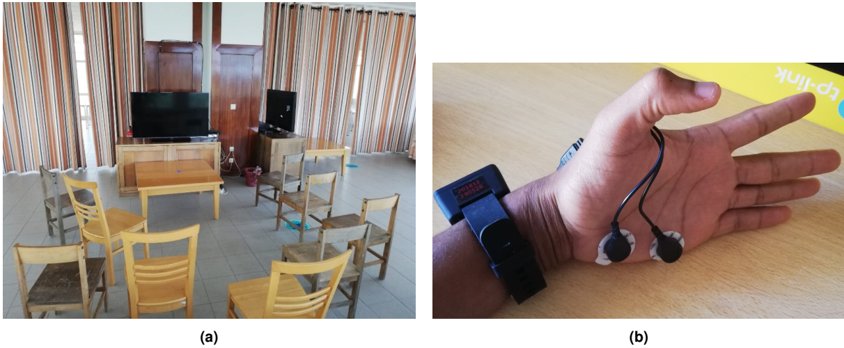
Figure 3.2: Experimental conditions of the acquisition process. (a) - Layout of the sitting area in relation to the LCD monitor. (b) - Device and electrode placement at the wrist and palm of the hand, respectively.
